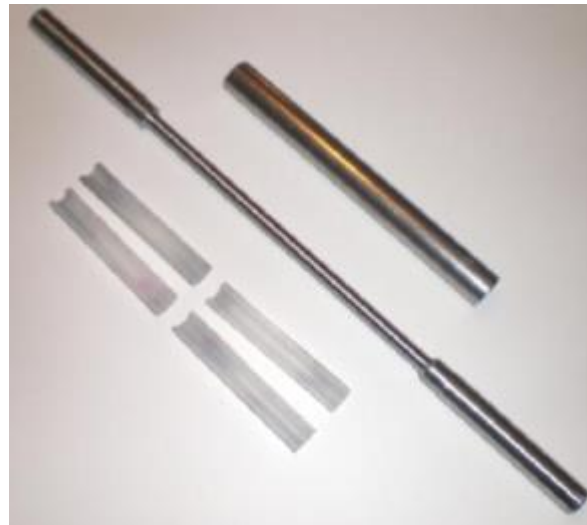
Fig. 4. Energy dissipating device: (a) local incorporation, (b) front view and (c) section view detail.
